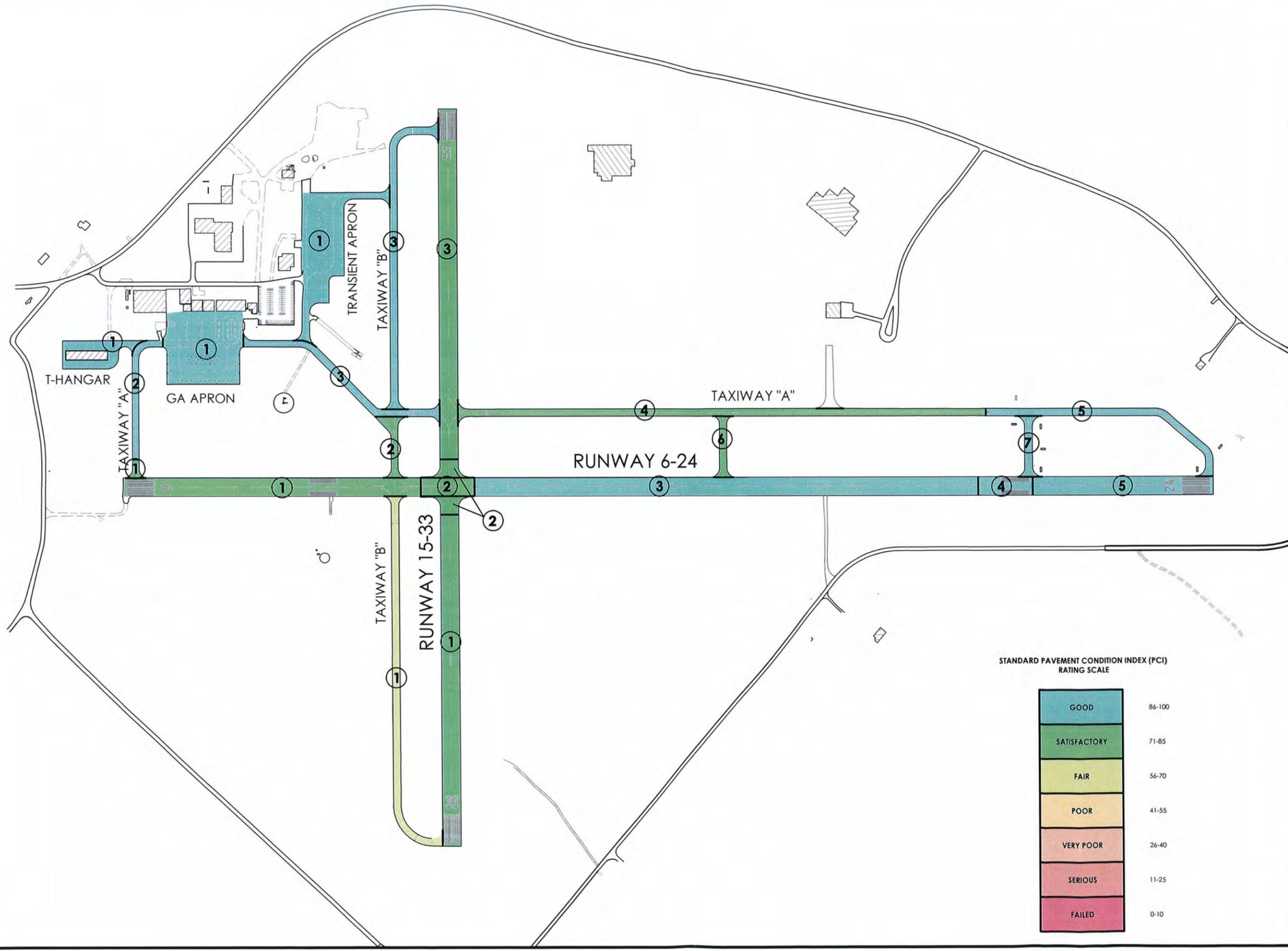
STANDARD PAVEMENT CONDITION INDEX (PCI)
